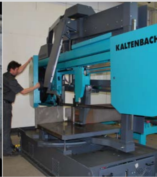
The retractable vertical clamping device enables easy, user-friendly blade changing in no time at all.
