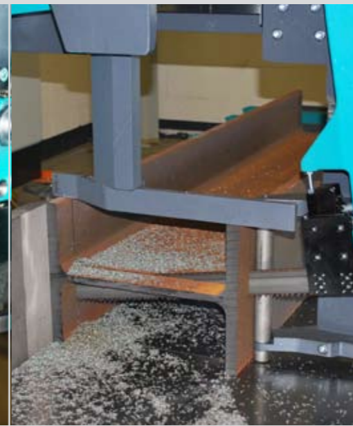
Vertical clamping device with tensioning blades for optimum grip of short pieces
