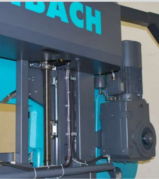
Increased cutting performance through the use of a ballscrew spindle for the sawblade feed.
