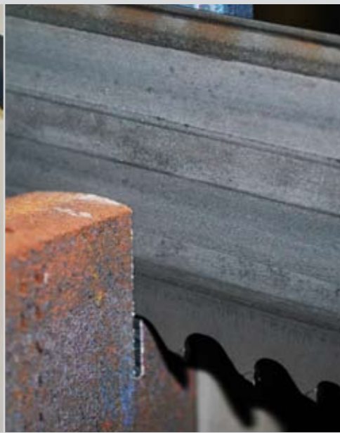
Carbide saw blades can be used for the first time, due to the powerful saw drive (12.9 kW) and AFC system, these increase cutting performance by fifty percent.
