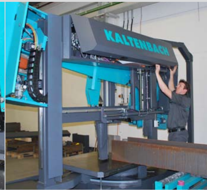
Good accessibility to electronics, hydraulics and atomised lubrication system.
